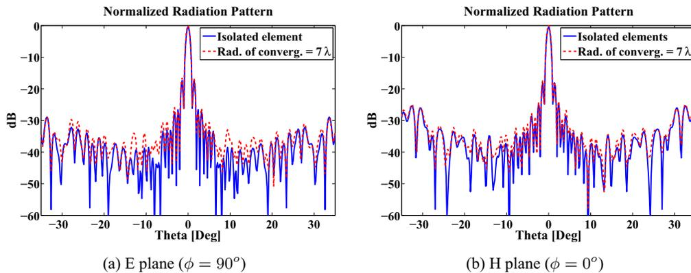
Figure 4: Array Patterns assuming isolated element patterns and including mutual coupling up to a  $7\lambda$  radius.
