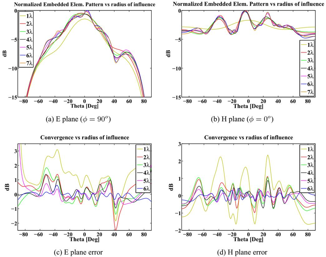
Figure 3: Embedded element patterns and errors for different radius of influence.
