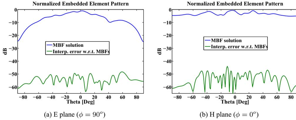
Figure 1: Embedded element pattern obtained with the MBF approach and error for the interpolation technique w.r.t MBF solution.
