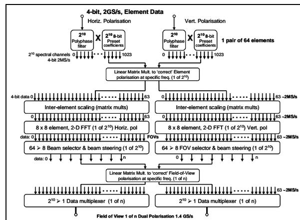
Figure 2. Processing for Beam-former Processor
