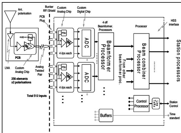
Figure 1. Signal flow in an all-digital system
