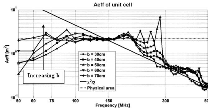
Fig. 4: Simulated unit cell effective aperture for an infinite regular array. The different curves are for different elements sizes. In the legend is the value of  $b$ . Also the  $\lambda^2/2$  curve is plotted together with the physical area of the unit cell.
