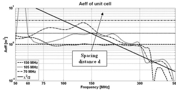
Fig. 3: Simulated unit cell effective aperture for an infinite regular array. The different curves are for different spacing distances between elements. In the legend is the frequency of the half wavelength spacing  $d$ . Also the  $\lambda^2/2$  curve is plotted together with the physical areas for each spacing  $d$ .
