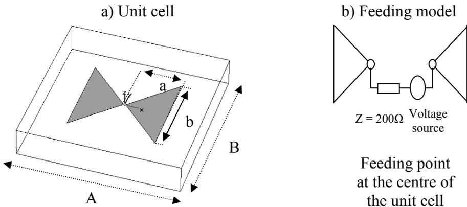
Fig. 1: Simulated unit cell of the regular array. a) Unit cell. The element type is a PEC made Bow-Tie element placed 166 mm on top of a ground plane. b) Feeding model.
