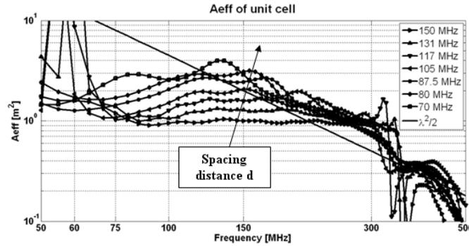
Fig. 2: Simulated unit cell effective aperture for an infinite regular array. The different curves are for different spacing distances between elements. In the legend is the frequency of the half wavelength spacing  $d$ . Also the  $\lambda^2/2$  curve is plotted.
