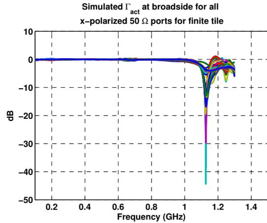
Fig. 8. Simulated single-ended active reflection coefficients for all  $x$ -polarized elements.
