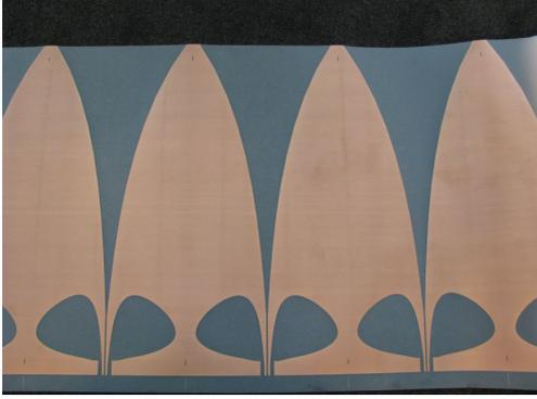
Fig. 2. Part of the foil with antenna elements.
