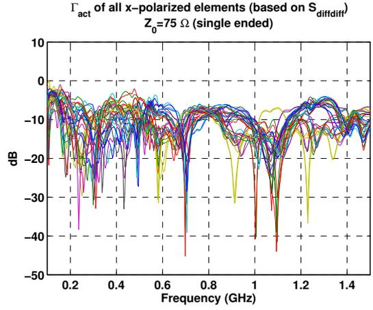
Fig. 4. Differential mode active reflection coefficient of all  $x$ -polarized elements at broadside.
