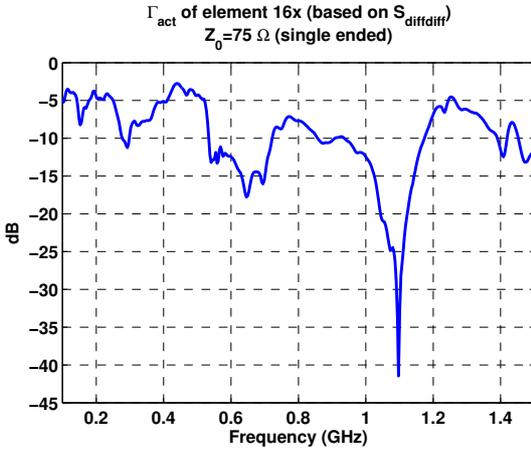
Fig. 3. Differential mode active reflection coefficient of one of the four center elements at broadside.
