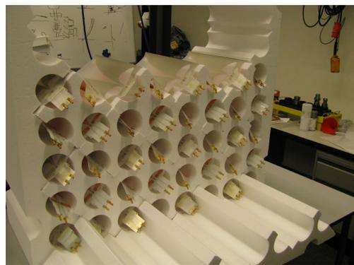
Fig. 1. The interior of the dual polarized Vivaldi array.
