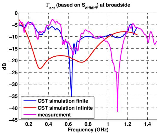
Fig. 7. Simulated differential mode active reflection coefficient of both a finite and an infinite array. The measured differential mode active reflection coefficient is shown as well.
