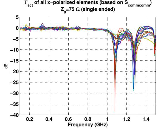
Fig. 5. Common mode active reflection coefficient of all  $x$ -polarized elements at broadside.
