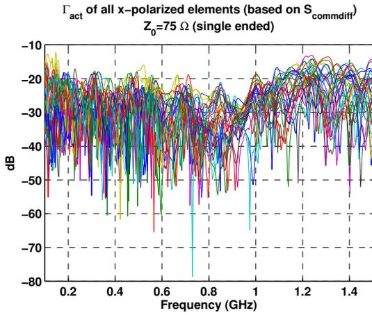
Fig. 6. Active reflection coefficient (based on  $S_{commdiff}$ ) of all  $x$ -polarized elements at broadside.
