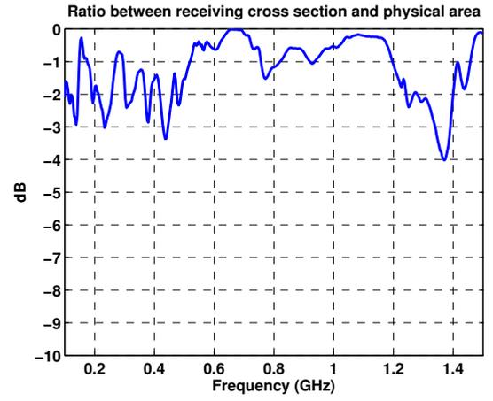
Fig. 10. Ratio  $A_{r,diff}/A_{ph}$  of one of the center elements for broadside as a function of frequency.
