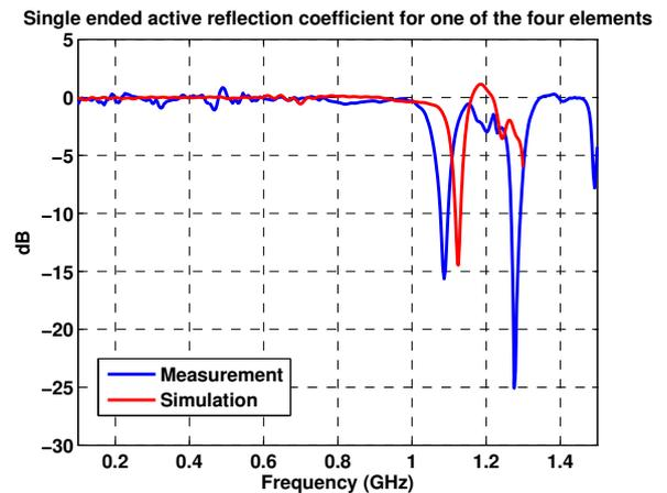
Fig. 9. Measured and simulated single-ended active reflection coefficient of one of the four center elements.
