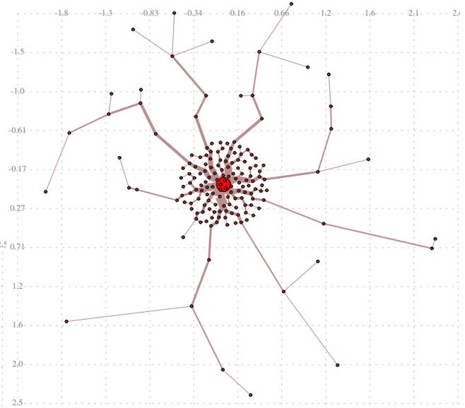
Figure 6: An example configuration of 165 collectors with a data rate of 2 TBytes/s each, consisting of a highly concentrated inner core of 1 km diameter and some sparse random distribution within 5 km diameter from the CB. The infrastructure was optimised for total trench and cable cost. Total cost is €748.82k, of which €395.27k are cable costs and €353.56k are trench costs.
