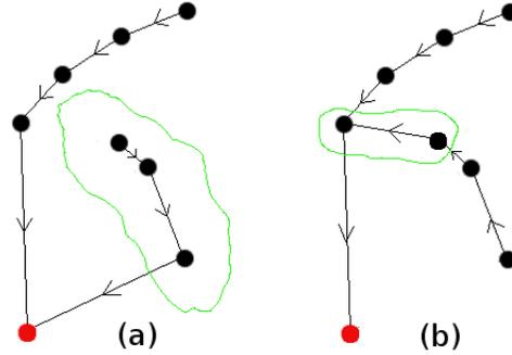
Figure 3: Example of *Reverse Lines* algorithm in action: the flow in a linear chain of connections is reversed (a), the most down stream link is disconnected and a more cost-effective connection is made at the up stream end (b).
