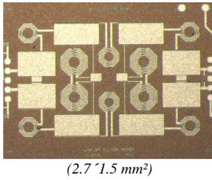
Fig. 3 Photograph of the balanced 5<sup>th</sup> order Tchebychev band pass filter
