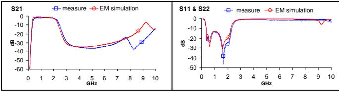
Fig. 2 Measurements and EM simulations of the single-ended filter
