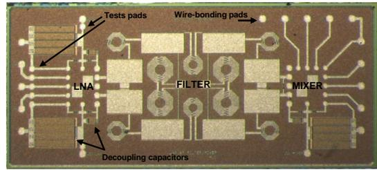
Fig. 7 Photograph of PICS substrate (5.2x2.3mm)
