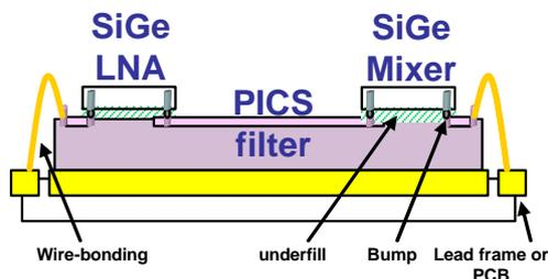
Fig. 6 Cross-section of the SiP
