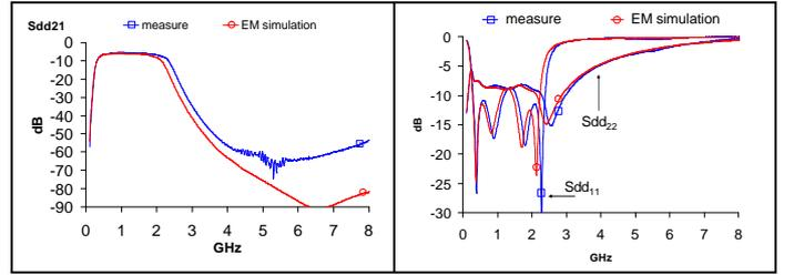
Fig. 4 Measurements and EM simulations of the balanced filter
