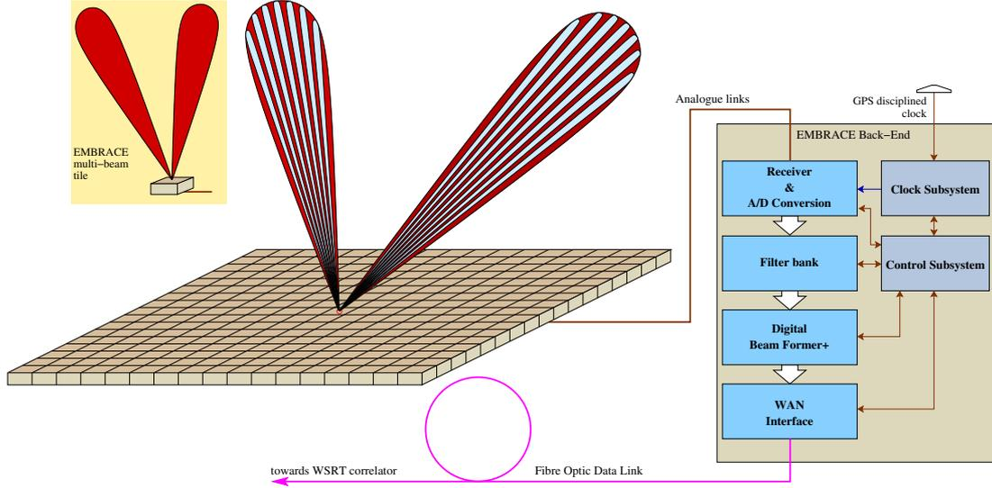
Figure 1: A system level block diagram of EMBRACE showing the formation of independent multiple fields-of-view at both the tile and station level, with processing at the back-end
