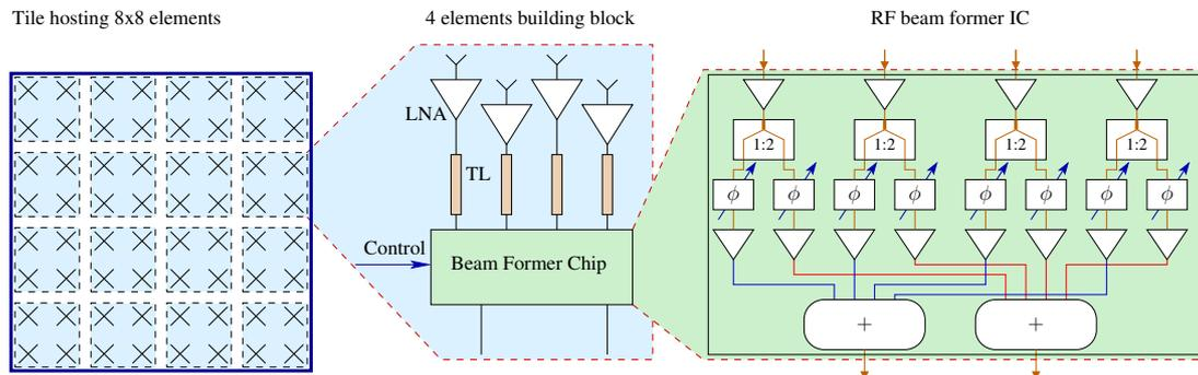
Figure 2: EMBRACE tile front-end architecture
