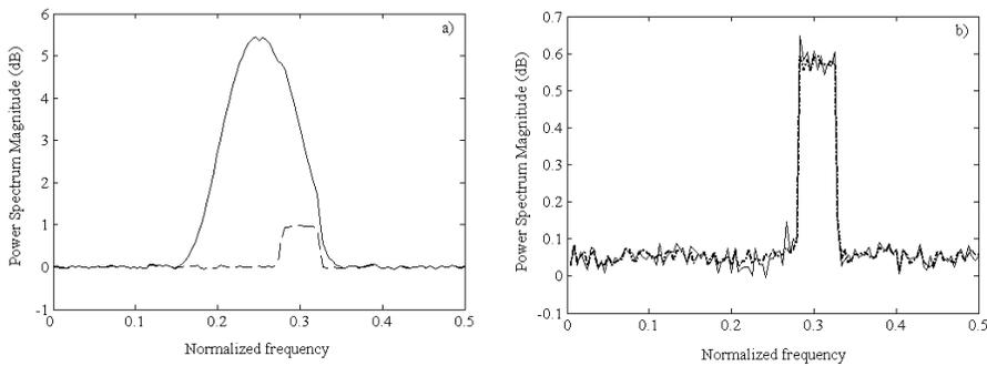
**Fig. 7.** Simulation with a continuous spread spectrum emission. a) Spectrum estimated without cyclic cancellation. The position of the simulated cosmic source is drawn as a dashed line – it cannot be detected through classical spectral analysis. b) Spectrum estimated with cyclic cancellation. The dashed profile is the expected one (Bretteil, 2005).
