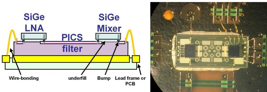
**Fig. 3.** *Left:* Cross-section of the SiP developed using PICS technology: the underfill is a non-conductive adhesive, which connects the whole surface of the active die to the substrate. It protects the inter-connection area from moisture, consolidates mechanical connections and improves thermal dissipation. *Right:* photograph of the SiP. Substrate dimensions: 5.2mm × 2.3mm
