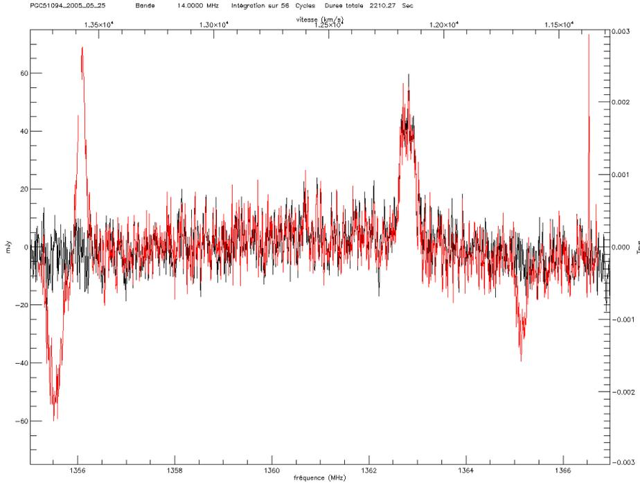
**Fig. 6.** Example of a real-time RFI mitigation system implemented at the Nançay Radio Telescope: redshifted 21-cm HI line of the galaxy PGC 51094 with (black) and without (red) radar blanking.
