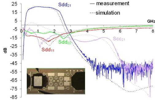
**Fig. 4.** SiP (LNA-filter) under test and its measurement results. Sdd21: differential mode gain; Scc21: common mode gain; Sdd11, Sdd22: input & output matching.
