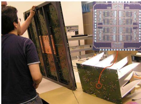
**Fig. 2.** The beam former chip developed by the Nançay microelectronics group integrated on the back of one of the EMBRACE tiles, with the densely packed Vivaldi antennas on the reverse side. The tile is about one square metre in size.
