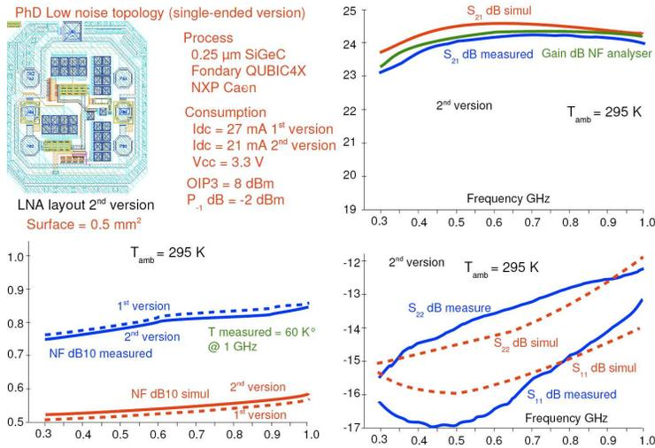
**Fig. 1.** Nançay design of a low noise amplifier for the lower frequency band 300-1000 MHz, which is expected for the planned european *Aperture Array Verification Programme* scientific demonstrator of dense aperture arrays for the SKA.
