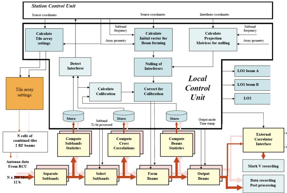
**Fig. 5.** An EMBRACE backend. Based on a LOFAR backend, the system has been reconfigured and the command and control system have been adapted for the EMBRACE design by the Nançay team.
