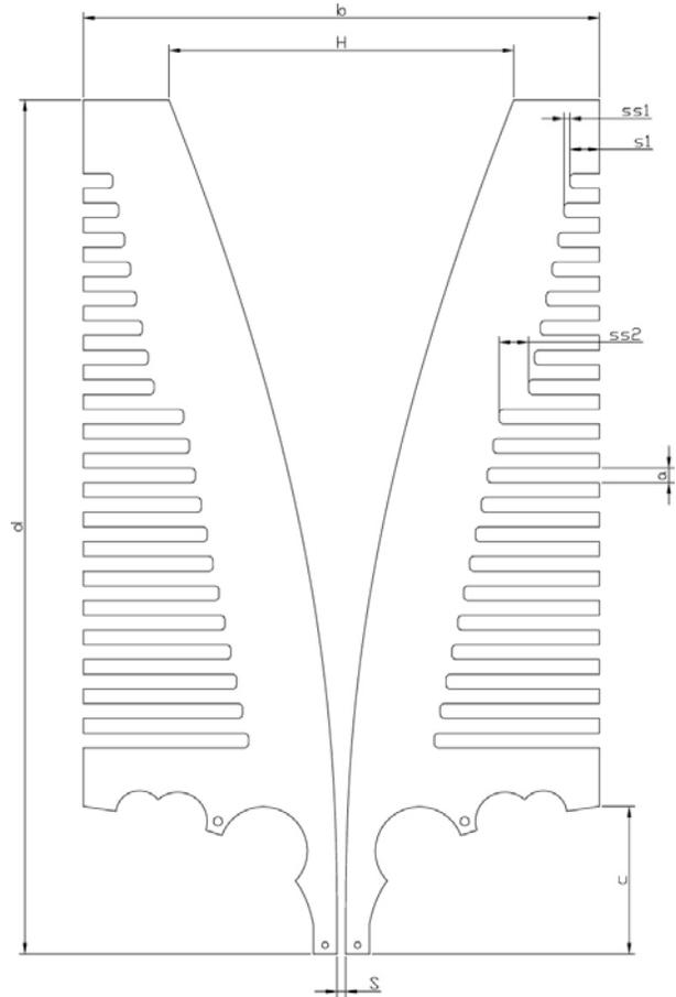
Fig. 3. The outline profile for the proposed BECA antenna, the width of the slotline at the end for feeding  $S = 3$ mm, the thickness of the conducting plate is 1.5 mm in the paper and therefore the characteristic impedance of the slotline at the feed point is 150 ohms. The characteristic input impedance can be tuned by changing the width of the slot and the thickness of the conducting plate
