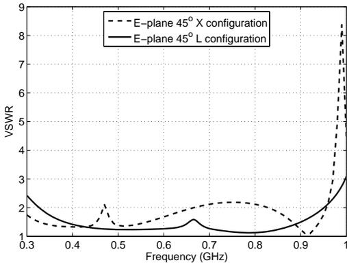
Fig. 5. The  $45^\circ$  in the  $E$ -plane scan performance for the dual polarized BECA array with a L and X configuration; The element spacing is 170mm, the depth of the element  $d = 280$ mm.
