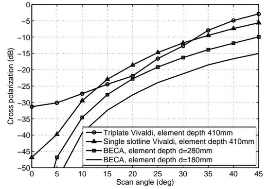
Fig. 6. The cross polarization performance comparison for scans in the  $D$ -plane at 1 GHz, it is based on infinite array simulation for dual polarized arrays, the elements for the three dual-polarized arrays share the same element spacing of 170mm, the element depth for Vivaldis is 410mm, the element depth for BECA is 280mm and 180mm.
