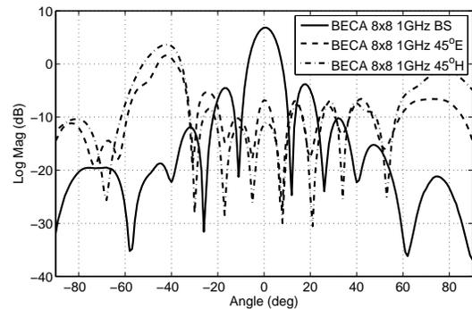
Fig. 9. The scanned array patterns of the  $8 \times 8$  subarray at 1 GHz in three directions: broadside,  $45^\circ$  in the  $E$ -plane and  $45^\circ$  in the  $H$ -plane.
