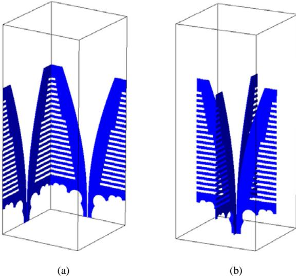
Fig. 4. The dual-polarized BECA unit cell for infinite arrays, (a) L configuration, the intersection is half the lattice spacing to the slotline, (b) X configuration, both elements share the same mutual axes and it is in the centre of the slotlines for both elements.
