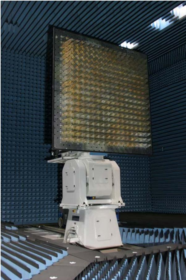
Fig. 7. The fabricated dual polarized  $16 \times 16$  BECA array, the dimension for the element is:  $b = 173.5\text{mm}$ ,  $d = 280\text{mm}$ ,  $S = 3\text{mm}$ ,  $c = 40\text{mm}$ ,  $H = 117\text{mm}$ ,  $a = 5\text{mm}$ ,  $sl = 10\text{mm}$ ,  $ss1 = 2\text{mm}$ ,  $ss2 = 10\text{mm}$ , the thickness of the conducting plate is 1.5 mm and therefore the element separation is 175 mm.
