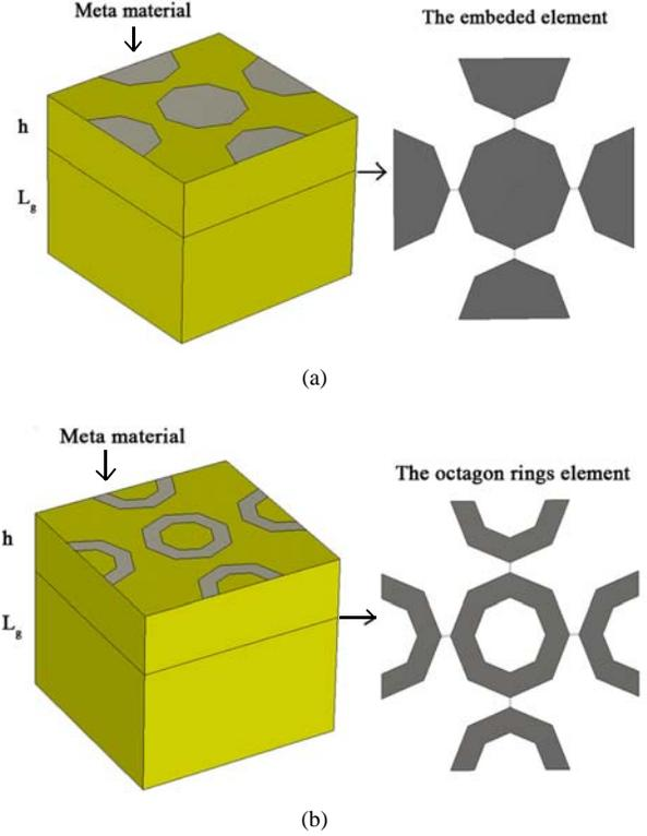
Fig. 3. The unit cell of the octagonal antenna, (a) Octagonal patches, (b) Octagon Rings Antenna.
