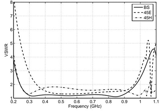
Fig. 7. Scan performance for an ORA,  $C=1\text{pF}$ ,  $h=70$  mm,  $L_g=110$  mm, the scale factor  $sf=0.94$ , the size of the unit cell is 165 mm.
