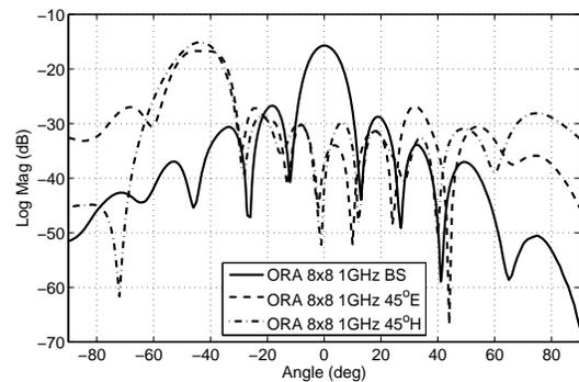
Fig. 13. Measured scanned beam pattern at 1 GHz for the finite ORA array.
