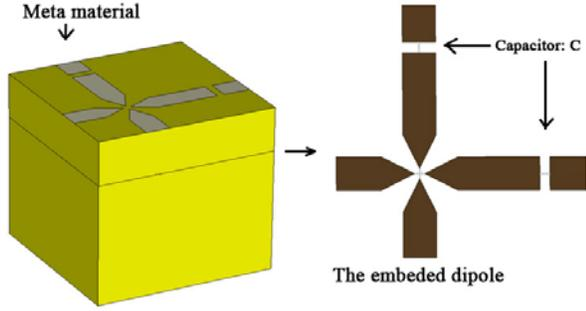
Fig. 1. The unit cell for a current sheet array with predetermined reflection conducting material on the top.
