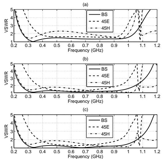
Fig. 4. The VSWR for the infinite dual-polarized arrays. (a) The square patch antenna array; (b) The circle patch antenna; (c) The octagon patch antenna.
