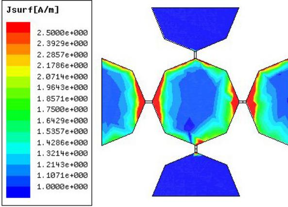
Fig. 5. The surface current at 700 MHz for broadside scan of an octagonal patch element in the infinite array.
