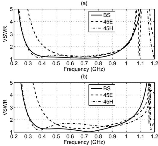
Fig. 2. The scan performance for an infinite current sheet dipole array, the element spacing is 150 mm, the distance from the array elements to the groundplane is 100 mm, (a) Two layers of dielectric material for reflection; (b) The displaced meta material for reflection, the distance from the array elements to the meta material layer is 40 mm.
