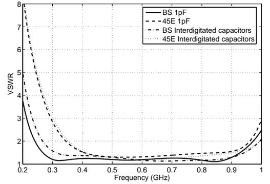
Fig. 8. The ORA with 1pF capacitor or interdigitated capacitors of 12 fingers,  $h=70$  mm,  $L_g=110$ mm,  $sf=0.9$  (a) 1pF capacitor; (b) Interdigitated capacitor with 12 fingers.
