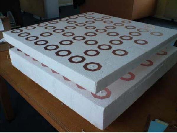
Fig. 6. The prototype of  $4 \times 4$  ORA finite array, the main element array is between the polystyrene foam slabs.
