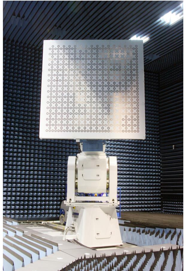
Fig. 10. The  $16 \times 16$  finite ORA array, photo courtesy SELEX Galileo.
