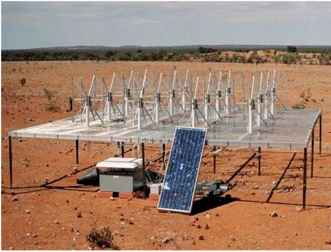
Fig. 3. An antenna ‘tile’ from the Mileura Widefield Array – Low Frequency Demonstrator (LFD), early deployment array. Each LFD tile consists of a 4×4 phased array of crossed dipoles. Image courtesy of the LFD Early Deployment team.
