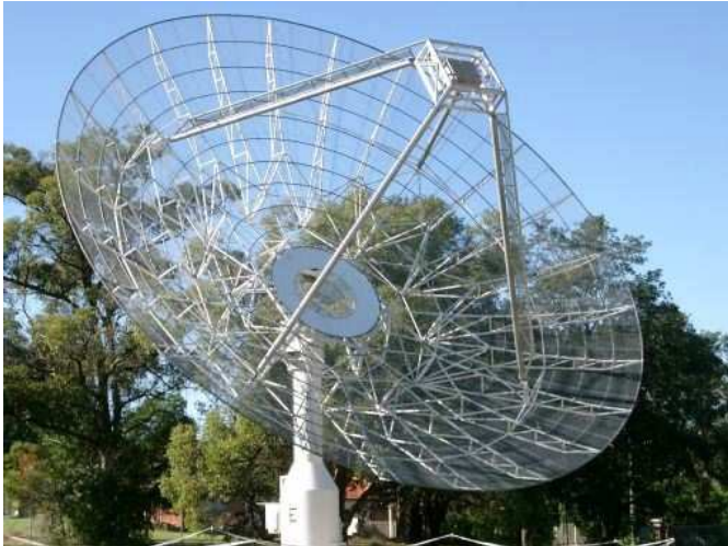
Fig. 1. The eastern antenna of the New Technology Demonstrator (NTD) located in Marsfield, Sydney. The NTD is a single-baseline interferometer designed to test Focal Plane Array (FPA) technology.
